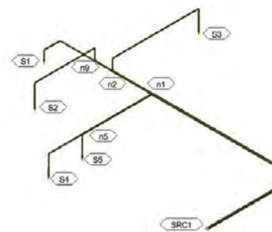
Any Revit sprinkler system may be traced and seamlessly delivered to the SprinkCALC / SprinkFDT software offering extensive calculation and reporting tools. Results are returned to your Revit project automatically, with tools to generate all code-required node labels, and to view and review most common hydraulic information right in the Revit model.
